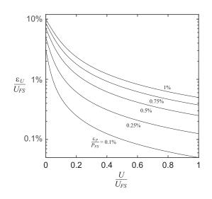
Figure 1: Relationship between uncertainty and velocity for a standard Pitot-static probe.
