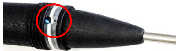
Figure 5: Correct alignment of modular system components
