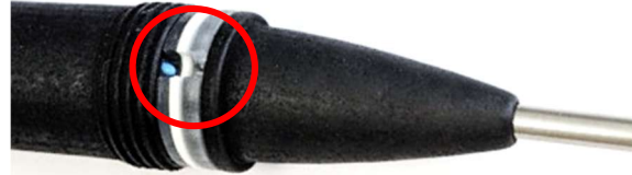
Figure 4: Correct alignment of modular system components
