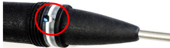
Figure 5: Correct alignment of modular system components
